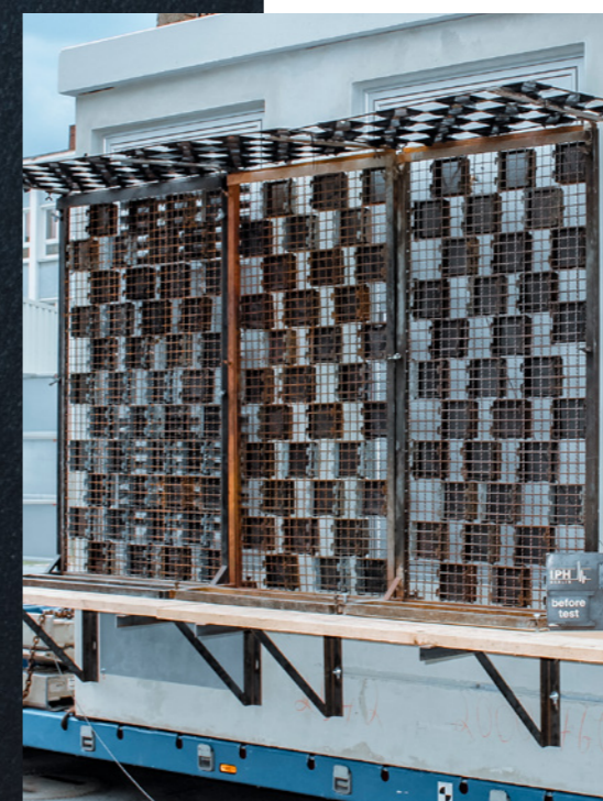
Internal arc fault test arrangement according to IAC-B 20 kA 1s for protection of the public
