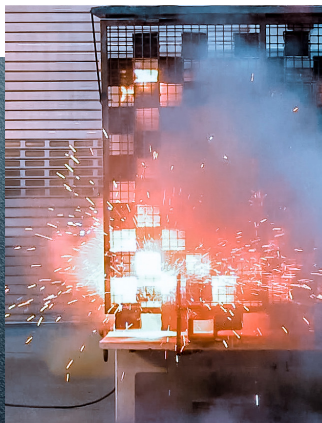
Internal arc fault test arrangement according to IAC-A 20 kA 1s for protection of operating staff
